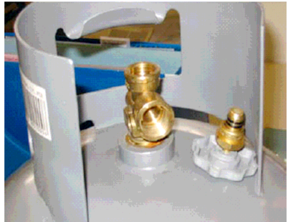
Valve can fall apart during closing action
